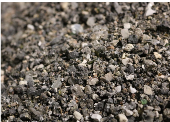
▲ Figs. 3 and 4: Iron-rich magnetic (right) and calcium-rich mineral (left) residual bottom ash from ZAV Recycling AG, as future raw materials in clinker production.
