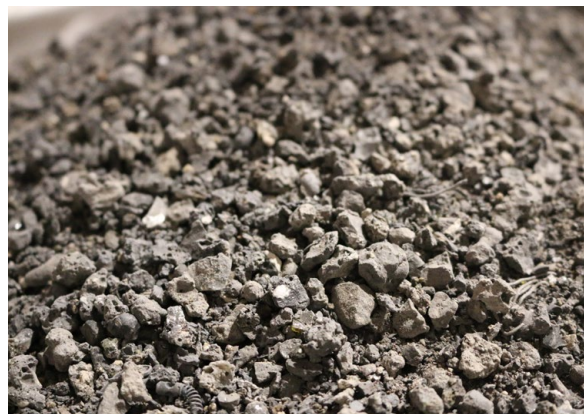
▲ Figs. 3 and 4: Iron-rich magnetic (right) and calcium-rich mineral (left) residual bottom ash from ZAV Recycling AG, as future raw materials in clinker production.
